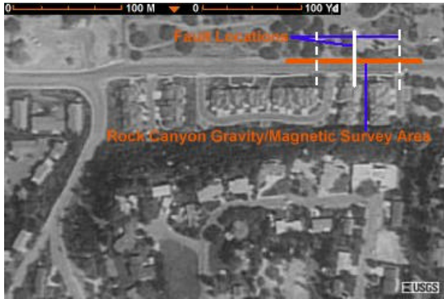
Figure 7: Aerial photo of the gravity/magnetic survey area showing possible fault locations
